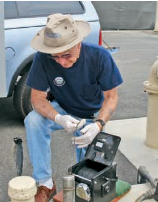
Obtaining water level at a Desalter II well.
